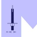
Material: Steel Finish: Pregalvanized Static Load Safety Factor: 3.5:1
